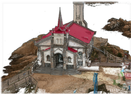
(A) Point cloud reconstructed by COLMAP
